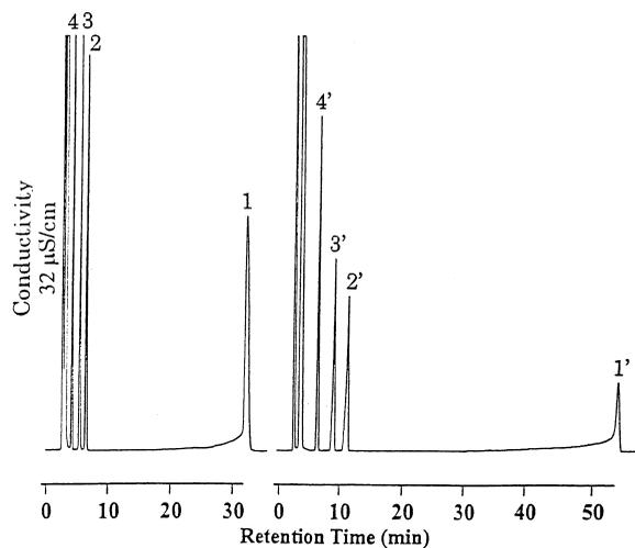
Fig. 5. Simultaneous determination of total acidity,  $\text{Ba}^{2+}$ ,  $\text{Mg}^{2+}$  and  $\text{Ca}^{2+}$  using iodide (left trace) and thiocyanate (right trace) as the counterions. Sample: 1.0 mM each of  $\text{Ba}^{2+}$ ,  $\text{Mg}^{2+}$  and  $\text{Ca}^{2+}$ ; 3.0 mM  $\text{H}^+$  (HCl). Other HPLC conditions as Fig. 1. Peaks: 1, 1' =  $\text{H}^+$ ; 2, 2' =  $\text{Ca}^{2+}$ ; 3, 3' =  $\text{Mg}^{2+}$ ; 4, 4' =  $\text{Ba}^{2+}$ .
