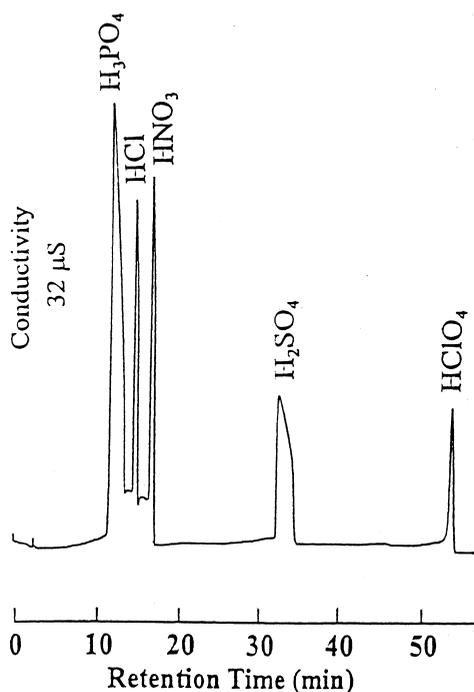
Fig. 2. Separation of a 20  $\mu$ l sample containing 10 mM concentrations of each of five acids. Conditions were the same as Fig. 1.
