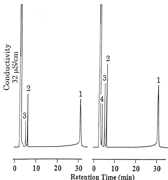
Fig. 6. Simultaneous determination of total acidity,  $\text{Ca}^{2+}$  and  $\text{Mg}^{2+}$  in hydrochloric acidic hot-spring water. The actual sample (left trace) and the sample after addition of 0.2 mM each of HCl,  $\text{CaCl}_2$ ,  $\text{MgCl}_2$  and  $\text{BaCl}_2$  (right trace). Peaks: 1= $\text{H}^+$ ; 2= $\text{Ca}^{2+}$ ; 3= $\text{Mg}^{2+}$ ; 4= $\text{Ba}^{2+}$ . Other HPLC conditions as Fig. 3.
