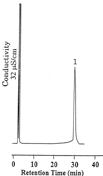
Fig. 1. Separation of 10 mM hydrochloric acid and 1.0 M sodium chloride on a silica  $C_{18}$  column (250×4.6 mm) coated with HDPC. Mobile phase was water alone at a flow-rate of 1.0 ml/min; 100  $\mu$ l sample, conductivity detection.
