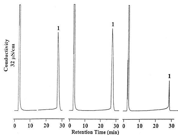
Fig. 4. Chromatograms of oxalic acid (left trace), tartaric acid (center trace) and ascorbic acid (right trace) with a 5-fold excess of sodium iodide added to the sample. Other conditions as in Fig. 1.
