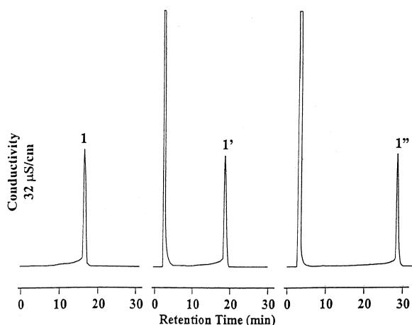
Fig. 3. Chromatograms of 2.0 mM HCl (left trace), 2.0 mM HCl with a 5-fold excess of sodium nitrate added to the sample (center trace), and 2.0 mM HCl with a 5-fold excess of sodium iodide. Eluent was water containing 10  $\mu$ M HDPC; conductivity detection.
